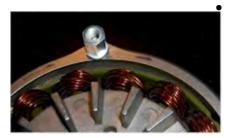
Then remove the central nut from the rotor and screw again the driver sleeve but tighten only slightly.
