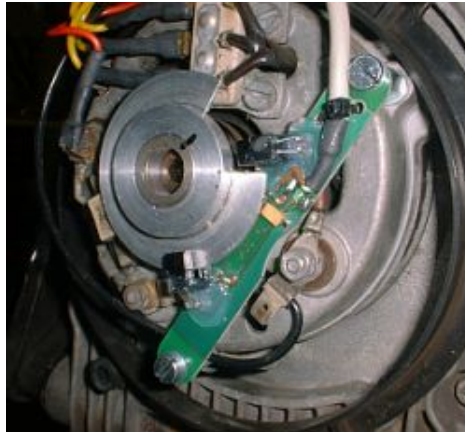
Installed pickup and sector disk
