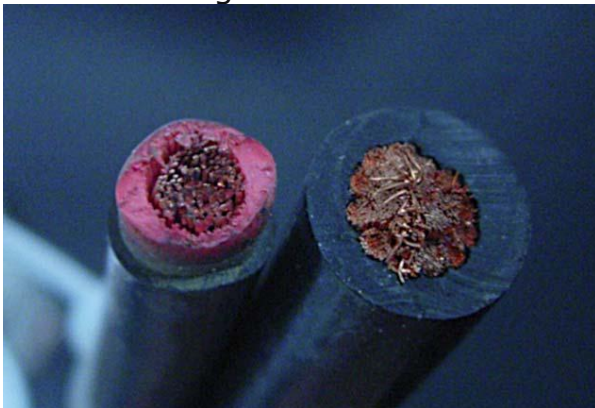
2&3) OEM starter lead on left, our 4 ga 1050 strand oxygen free copper lead on the right
